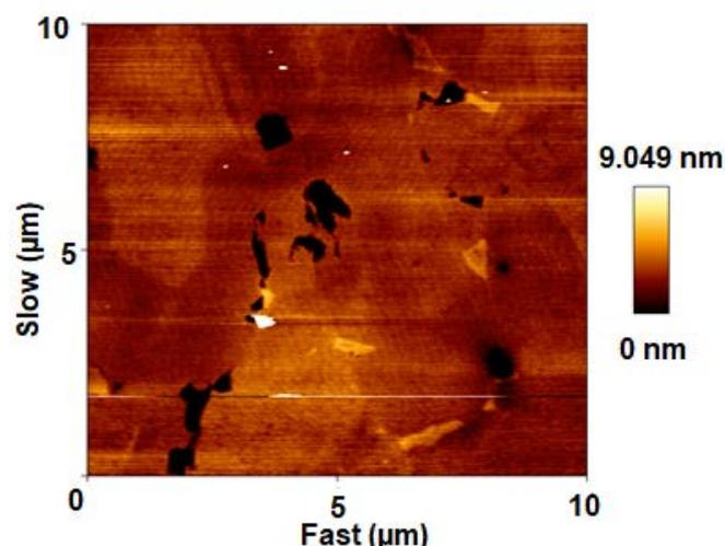
**Figure 1.** Topography of TiAlV surface with mirror-like finish.
