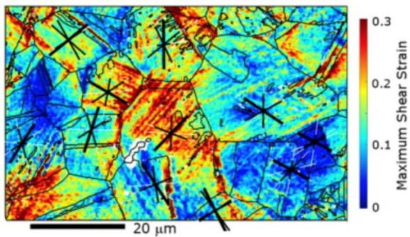
**Figure 2:** Strain distribution within crystals as a result of martensitic transformation [5].
