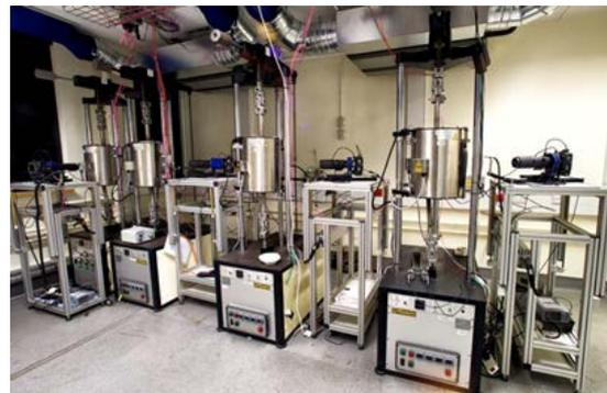
**Figure 1:** Creep testing facility at OU
