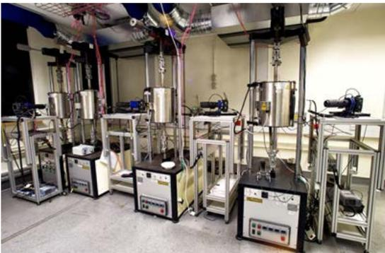
**Figure 2:** DIC-Creep testing facility at OU
