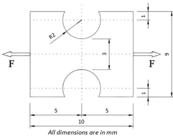
**Figure 1:** Miniature waisted-specimen to be used in VFM analysis. (Adapted from [1])
