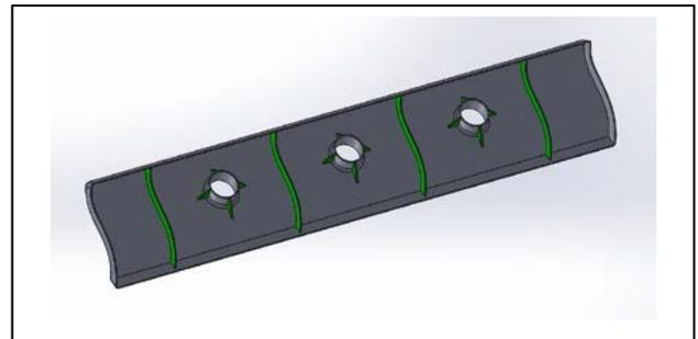
**Figure 1:** Example application of hybrid AM and thermoforming: Vehicle interior trim panel showing thermoformed component in gray and AM features in green
