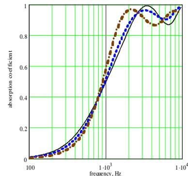
Figure 1 Target absorption spectrum (continuous line - porosity 0.95, flow resistivity 40 kPa s m<sup>-2</sup>, viscous characteristic length 50 μm, thermal characteristic length 150 μm, tortuosity 1.3, layer thickness 0.02 m) compared with spectra predicted for 1.9 cm layer of identical slit pores (broken blue line- slit width 80 μm, inclined at 40° to the normal) and 2 cm thick layer log-normal distribution of slits with mean width 36 μm (dash-dot brown line).
